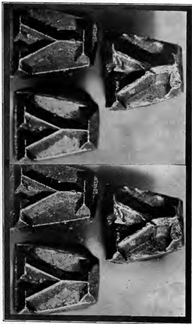
FIG. 202.—Stereoscopic photo-micrograph of the faces of typewriter type, showing the effect of wear and accidents, by which the work from such a machine can be positively identified. One letter new and unused, one showing one "scar" and one much battered. Some detail is lost in the process of engraving. This illustration and the other stereoscopic views are printed on a detached sheet at the end of the book.
